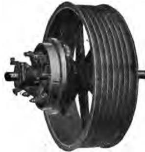
FIG. 142.—Pulley used for Rope Drawing.
